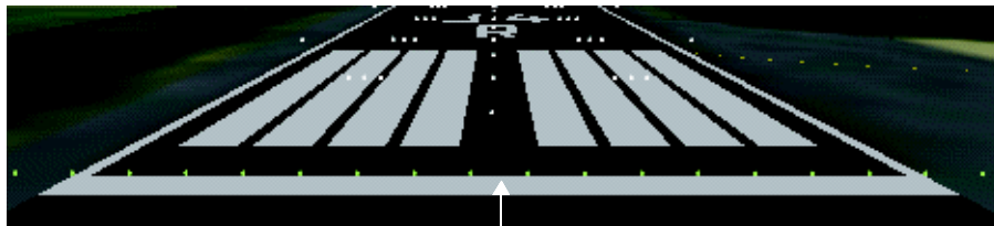
Runway end lights are green on the approach side (front face)
