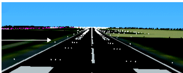
Runway edge lights
